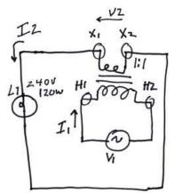
"Not really," said Hambone. "A critical bit of information is that the lamp is burning at normal brightness. That means it's receiving its rated voltage of 240 volts. That means the transformer's secondary voltage, V2, equals 240 volts. But there is more. That drawing shows the transformer's turns ratio is 1:1."
