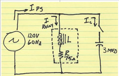
can see the power supply current was definitely lower with the switch closed," said Hambone as he sketched the circuit on Elmer's yellow pad.
