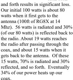
Our RG8X coax loss with 1:1 SWR would have been 20 watts. With the 3.5:1 SWR our loss increases to 34 watts (1.8db).
